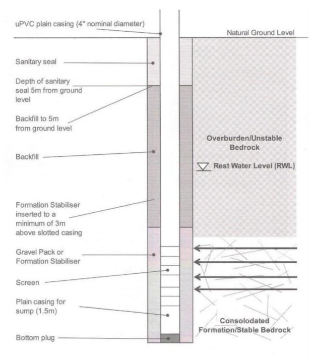
**Note:** In this typical borehole drawing (not to scale) the PVC casing & screen Nominal diameters should be 6" and not 4" as shown in the figure
